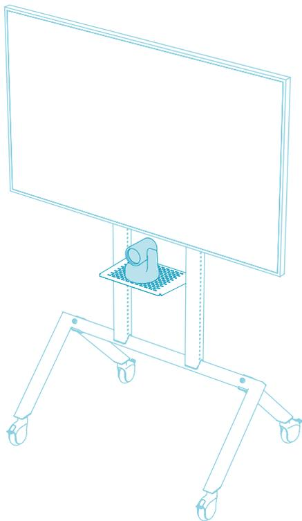
Note that the center slots include 1/4" clearance holes for camera mounting.
