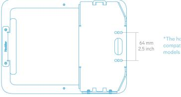
\*The hole pattern is compatible with previous models of Side Mount.
